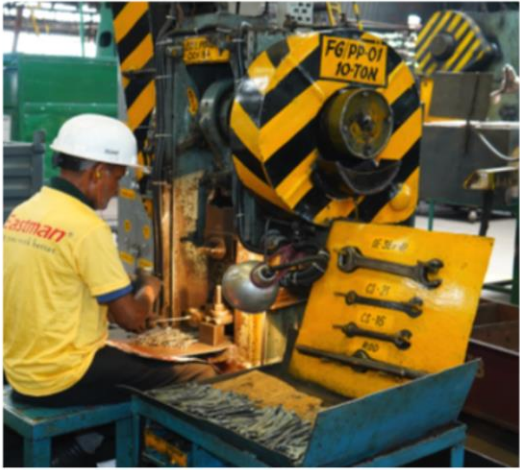
TRIMMING PRESS Removing extra flesh with accuracy
