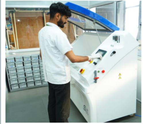
SALT SPRAY Checking the corrosion resistance of coatings and materials
