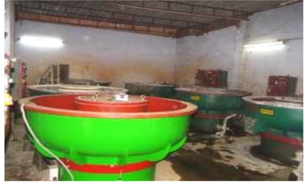
VIBRATORS FOR SPARKLING FINISHING Superior finish by Vibro polishing machines
