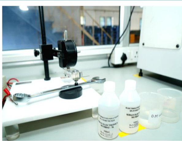
ELCOMETER Destructive type Compact and sophisticated thickness tester for the measurement of plating thickness
