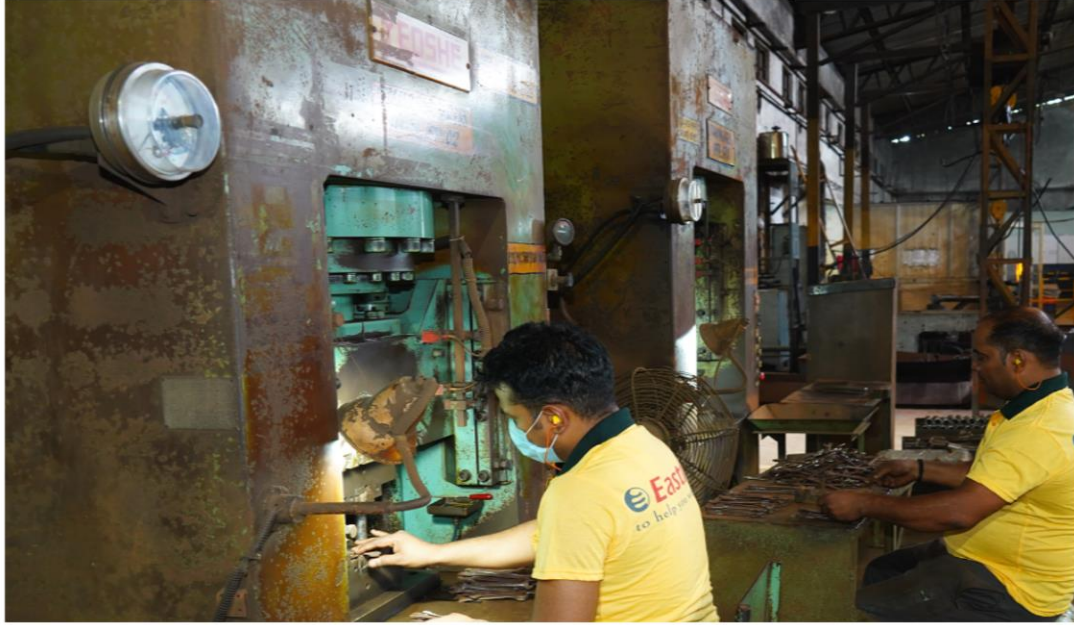
COLD STAMPING – BRANDING 200 + 400 ton Hydraulic press for brand Embossing by cold forging.
