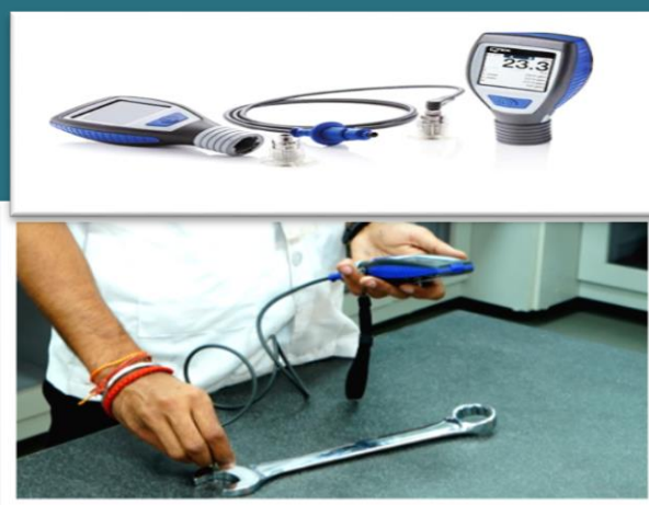
COATING TESTER Coating thickness tester (Nickel , Chrome, Zinc, Paint, Powder coating, Phosphate etc.)
