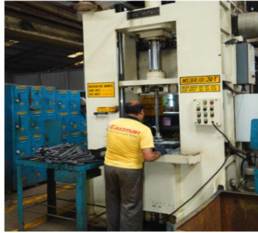
BROACHING Jaw accuracy is achieved by Hydraulic Broaching
