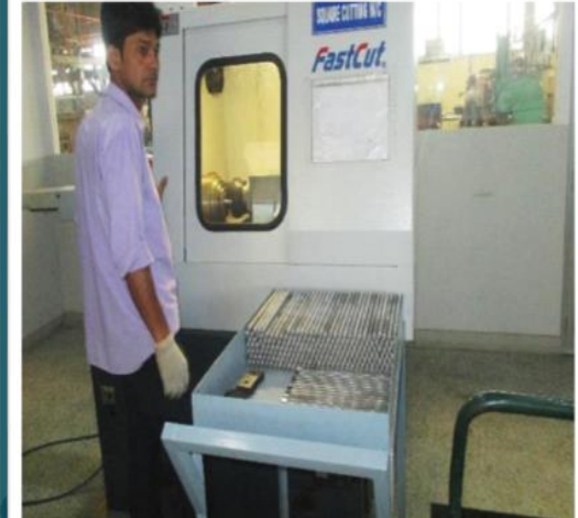
SQUARE CUTTING MACHINE Cuts all kinds of Shapes
