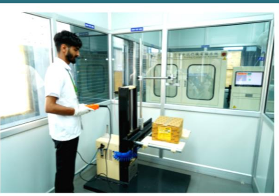
CARTON DROP TESTING Drop test of carton for checking Strength
