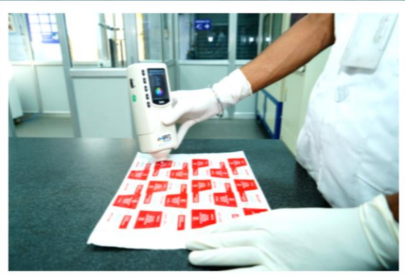
COLOR METER Checking printing color variations
