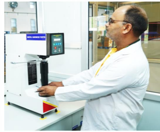
ROCKWELL HARDNESS TEST Digital hardness testing machine for quality assurance
